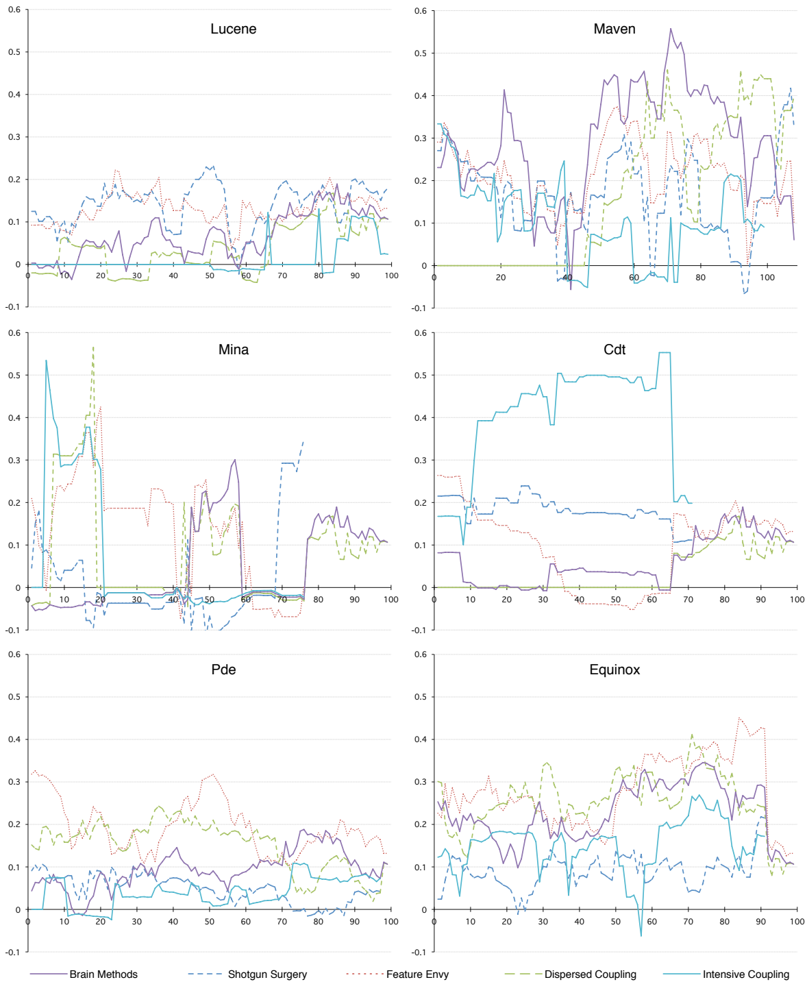
Fig. 7. Spearman's correlations between number of design flaws and number of post release defects over multiple versions of software systems.
